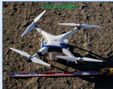
(U) Phantom 4 COTS Drone modified to drop IED Source: Conflict Armament Research
